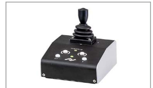
Motorized X-Y adjustment and component rotation.
