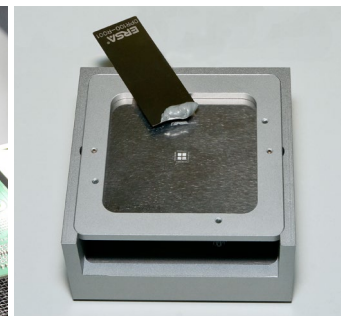
Dip&Print Station with "MLF32" stencil
