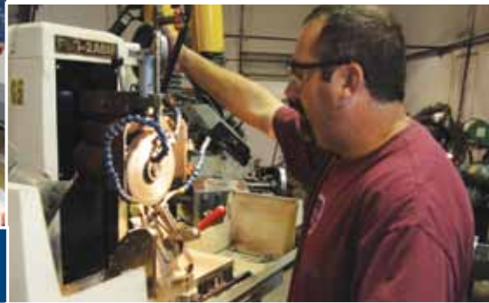
Surface grinding at Tronex insures exceptionally sharp cutting edges.
