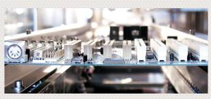
The systems are equipped with electrically width-adjusted conveying systems and center support.
