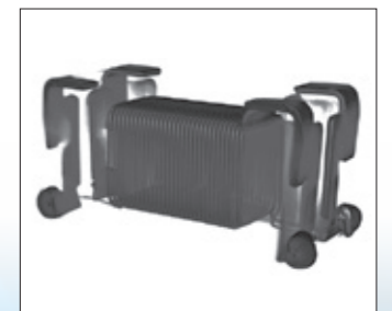
Reconstruction of a 4mm long inductor package
