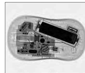
X-ray inspection image of a computer mouse
