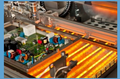
Perfect preheat concept with dynamic lower and upper preheaters
