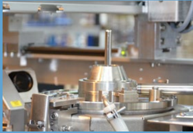
High single solder nozzle with a narrow diameter – ideal for solder joints between high components
