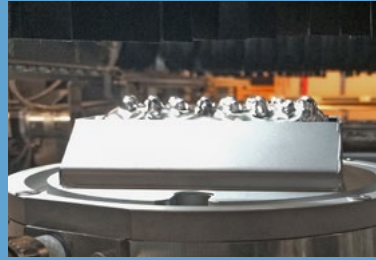
MINI-VARIO-WAVE solder nozzle for optimized throughput
