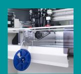
Intelligent feeders in all common sizes. Component spectrum from 01005 to 100x150 mm, component height up to 15mm
