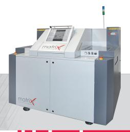
The **X3** is an automatic X-Ray inspection system featuring combined Transmission and 3D Technology for sophisticated high-speed inspection in electronic production. The system is based on the motion concept of the MatriX X2.5 AXI system. A newly developed 3D reconstruction software generates slice images for 3D analysis of solder joints. Main applications are double-sided boards with critical overlapping areas.
