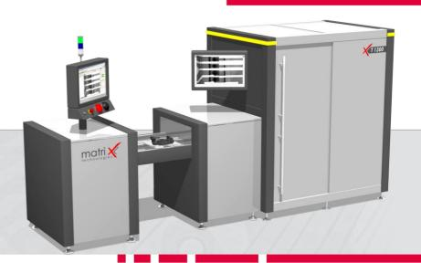
The **XT-1300** is an automatic x-ray inspection system, especially designed for the fully automatic inspection of high modules and complete assemblies. The system is equipped with a maintenance-free 130kV microfocus x-ray tube and a flexible carrier system that can be easily adapted to customer specific applications. The integrated test library includes algorithms for standard SMD joint inspection as well as for the inspection of joints on flexible circuit boards.
