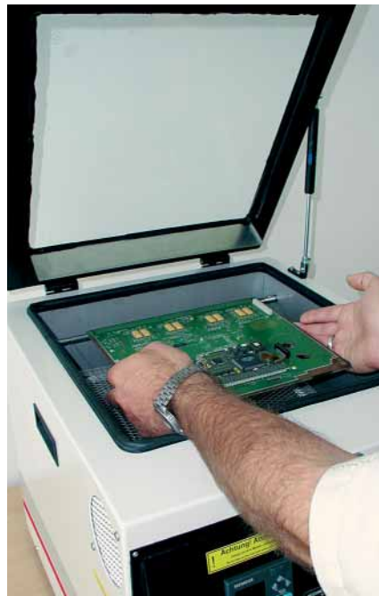
Entering the assembly into the process area
