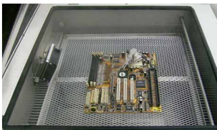
Work-piece carrier in feed-in position with assembly and desoldering unit
